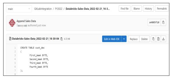
Use the committed FE script to generate a physical schema in your database. To generate schema, copy the FE script from your Git repository and run the script in the database.
